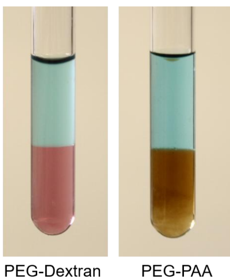
Figure 4.6 Images of phase-separated PEG-Dextran and PEG-PAA ATPSs in a test tube, with their appropriate colorimetric indicators for each phase. In the PEG-Dextran ATPS, red-colored BSA-GNs indicate the bottom dextran-rich phase and Brilliant Blue FCF dye indicates the top PEG-rich phase. In the PEG-PAA ATPS, brown-colored PAA-coated iron-oxide nanoparticles indicate the bottom PAA-rich phase and Brilliant Blue FCF indicates the top PEG-rich phase.
