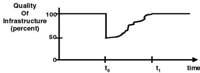
**Figure 6.5: Measure of seismic resilience—conceptual definition (Bruneau, 2003)**
