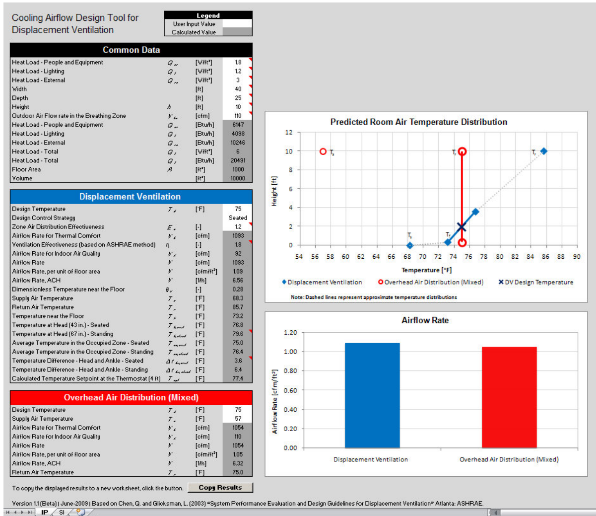
Figure 1 Displacement ventilation design tool (IP units).
