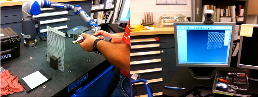
Figure 3. Scanning of expanded metal mesh layer using coordinate measuring machine.
