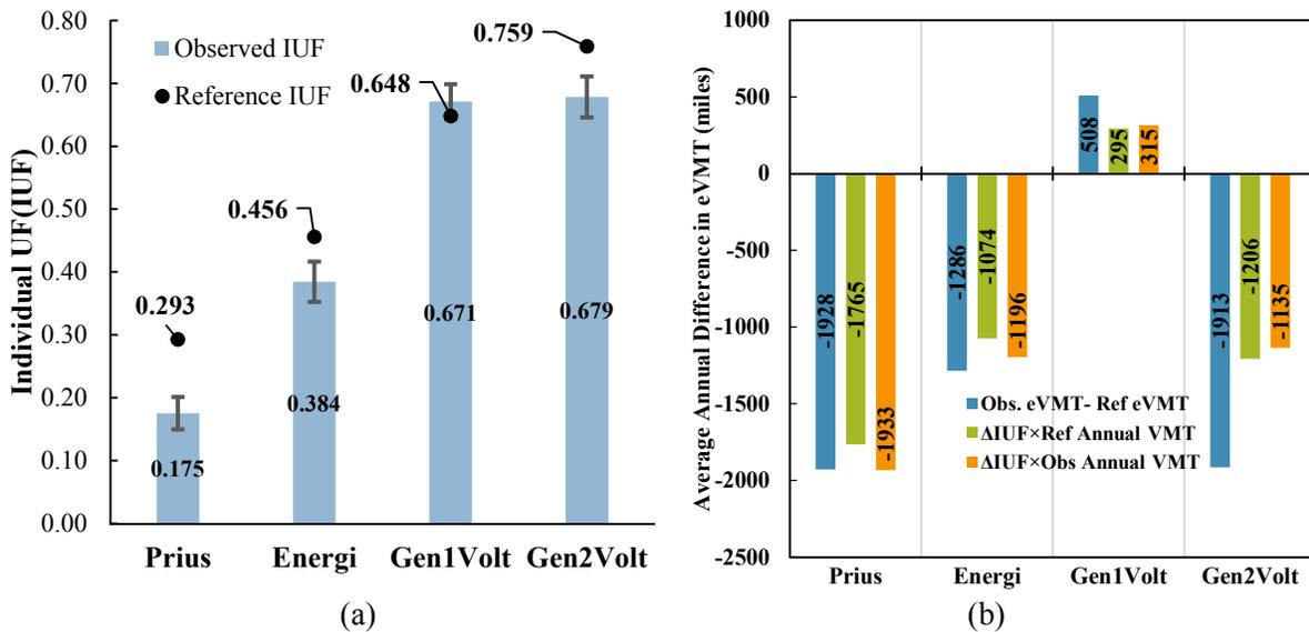
Figure 2.4 (a) Average observed IUF and J2841 IUF; (b) Annual eVMT differences between observed and J2841 estimates. Observed IUF are vehicle weighed average definition.
