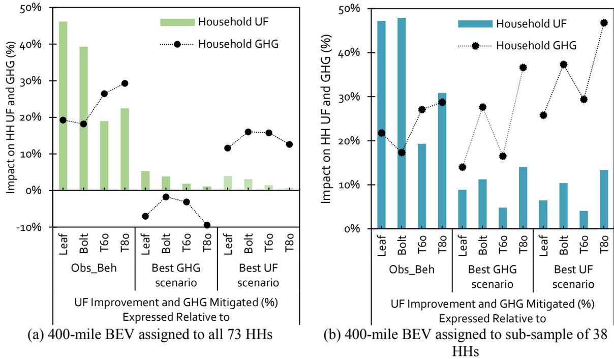
Figure 4.7. Effect of upgrading to 400-mile BEV on UF and GHG. Percentage change in UF and GHG expressed relative to observed behavior, best GHG and best UF scenarios. (a) Entire sample of 73 HHs upgrade to 400-mile BEV; (b) Sub-sample of 38 HHs upgrade to 400-mile BEV.
