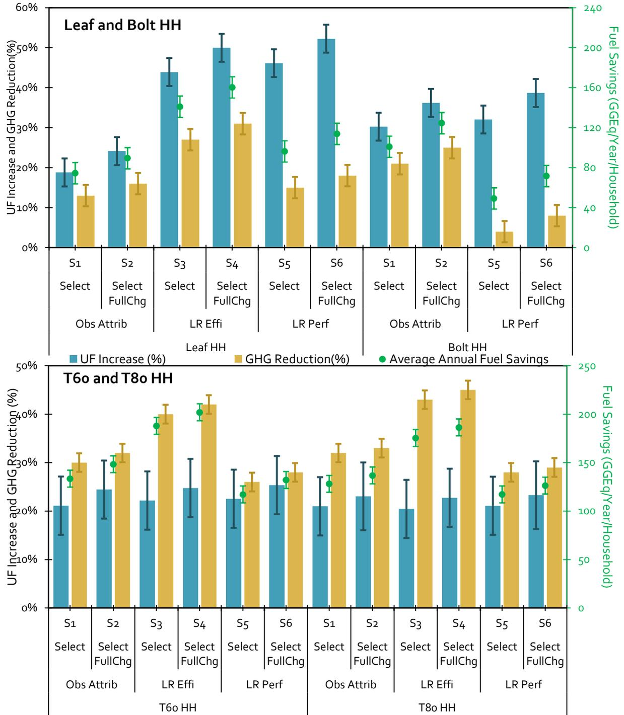
Figure 4.6. Percentage change in household UF and GHG (primary Y-axis) and average annual fuel savings in GGEq (secondary Y-axis) relative to *Obs\_Beh.* 33.7 kWh/Gallon gasoline equivalent[197].
