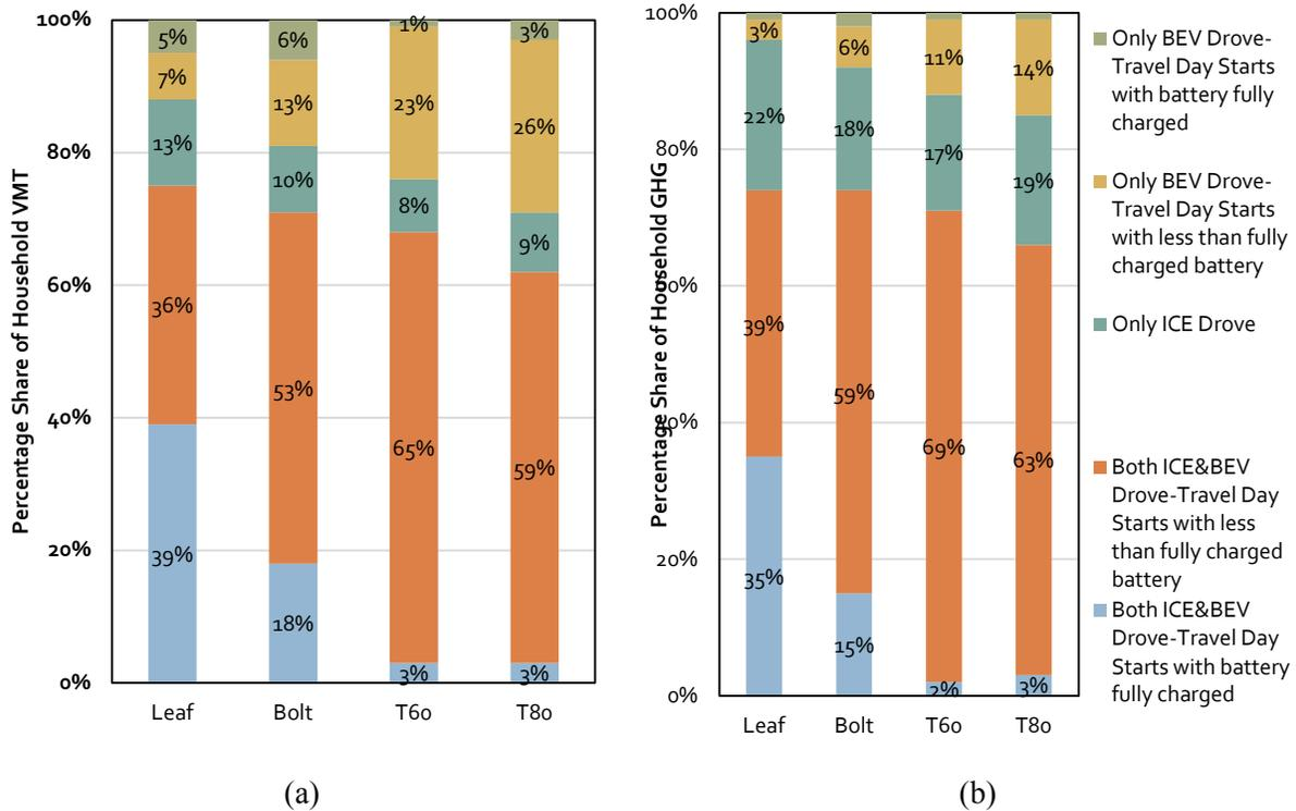
Figure 4.4 Observed HH VMT allocation and GHG contribution by type and number of vehicles used, and travel day starting SOC of the BEV. (a) Observed HH VMT allocation and ; (b) contribution to HH GHG. The type of day was chosen to be along the same lines as the scenarios.
