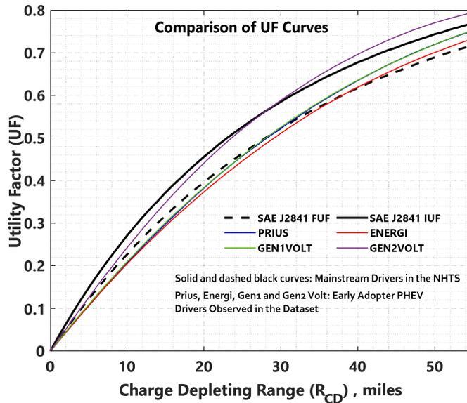
Figure 2.5 Comparison of J2841 UF curves (truncated) generated using NHTS/J2841 estimates and observed PHEVs
