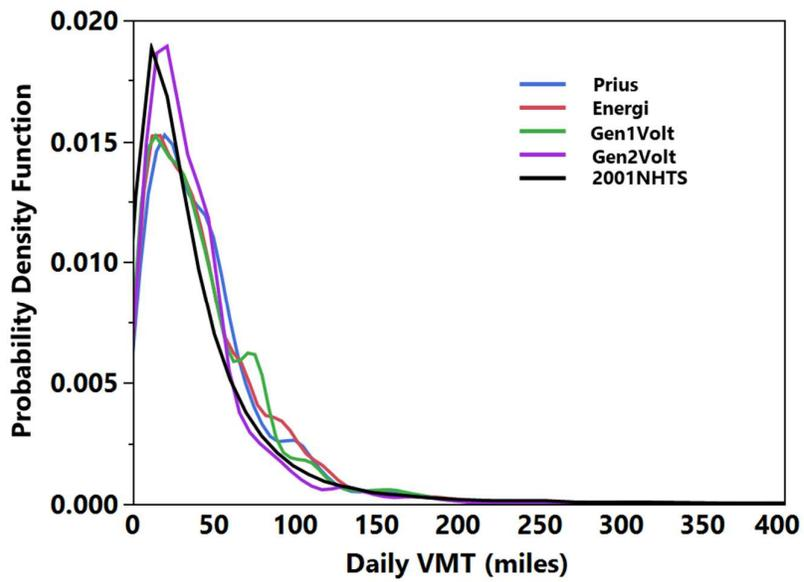
Figure A2. Expanded PDF plot of observed PHEVs and NHTS
