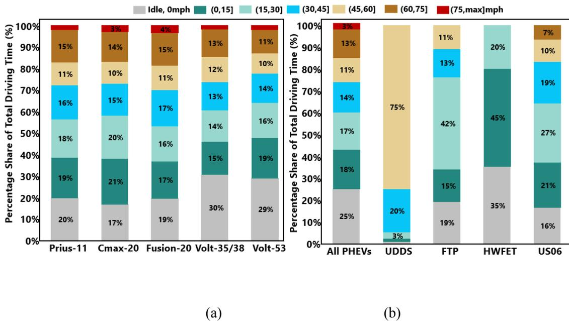
Figure 3.3 Percentage share of total driving time by driving speed in mph: (a) Observed PHEVs; (b) Comparison with EPA Test Cycles
