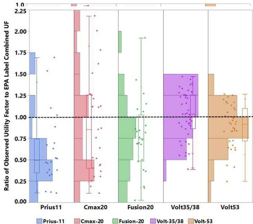
Figure 3.2. Ratio of observed UF to EPA label city/highway combined UF by PHEV model. Values above one indicates observed UF of PHEVs exceeded EPA estimates
