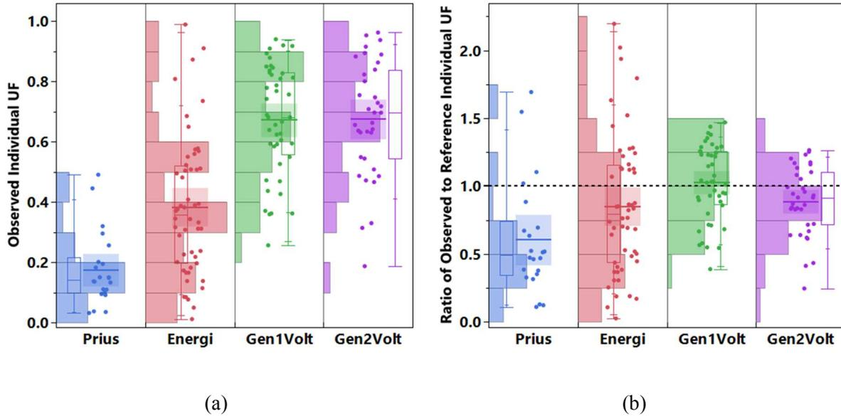
Figure 2.3 (a) Distribution of observed UF of every vehicle in the dataset; (b) Distribution of the ratio of observed UF to J2841 IUF
