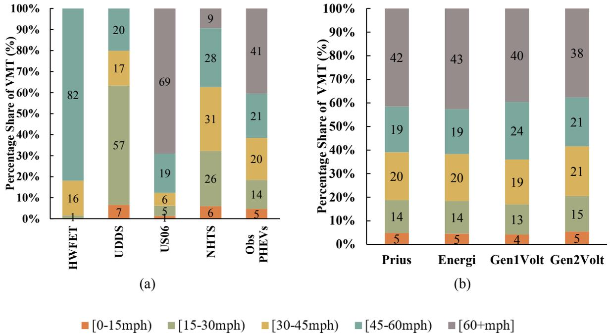
Figure 2.12 (a): Percentage share of VMT comparison between test cycles, observed PHEVs and NHTS by speed bins; (b): Percentage share of VMT comparison by speed bins
