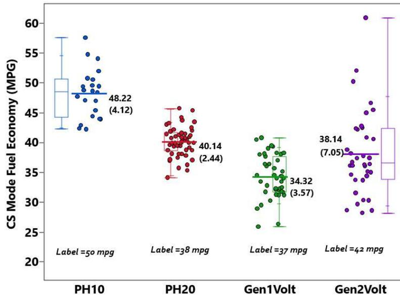
Figure 2.14 Distribution of observed PHEV charge sustaining mode fuel economy (mpg). Standard deviation shown within parentheses below the mean values and label values shown inset.
