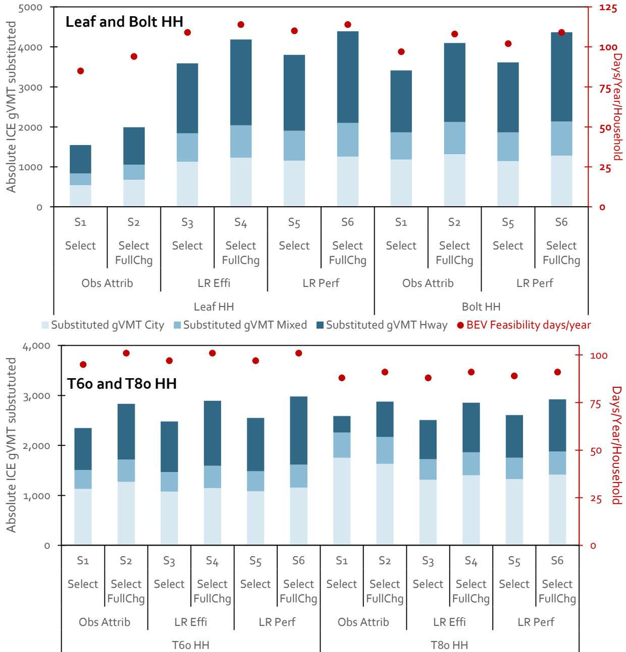
Figure 4.5. ICE gVMT substituted by driving style(primary Y-axis) and BEV feasibility in days/year/household (secondary Y axis).
