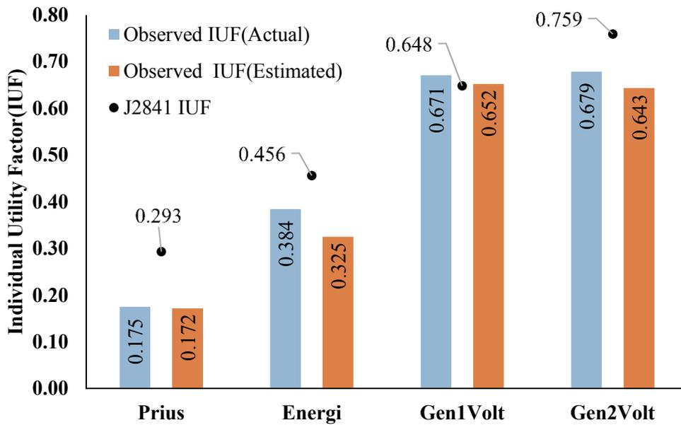
Figure 2.16. Comparison of actual IUF and IUF estimated alongside the reference J2841 IUF. Observed IUF are vehicle weighed average of UF by definition of IUF. Estimated and observed IUF are average values.
