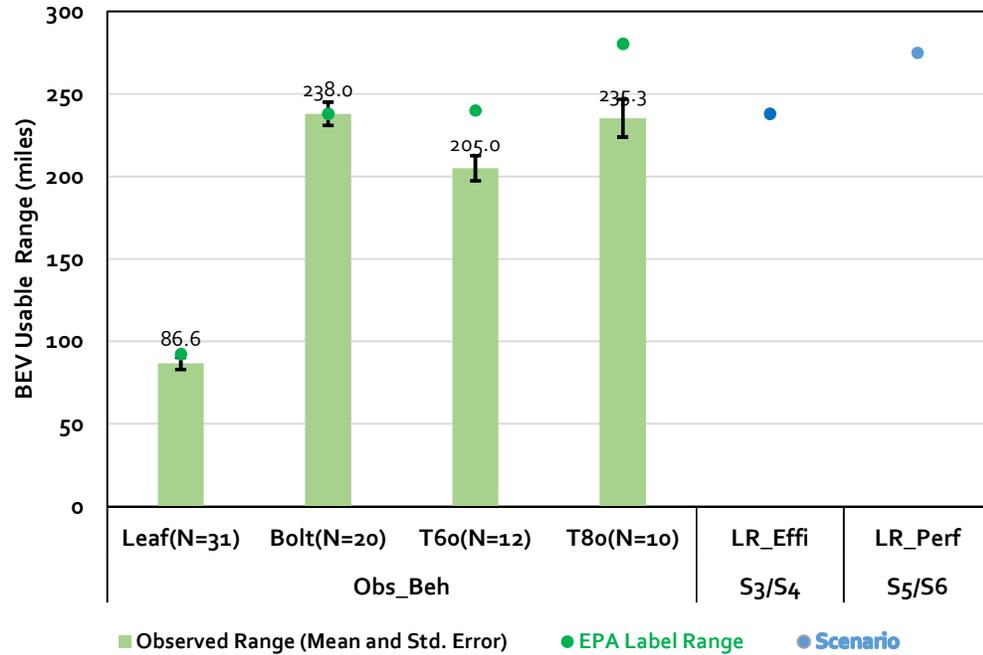
Figure C-3. Observed and EPA label range[88] (miles) of the BEV by driving styles. Light green columns and the black bars depict the mean and standard error of observed range. Dark green dots are the EPA label average fuel economy. Blue dots show the upgraded range for *S3 LREffi* and *S4 LREffi FullChg* and *S5 LRPerf* and *S6 LRPerf FullChg* scenarios.
