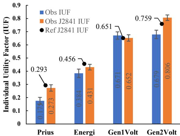
Figure 2.6 Means and std. error of Observed IUF, observed IUF after applying J2841 UF method, and reference J2841 IUF.
