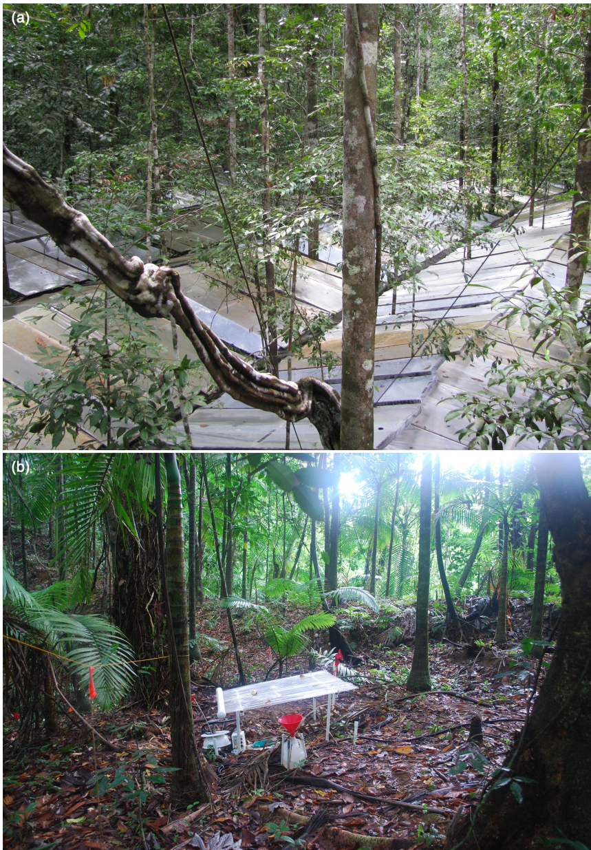
Figure 1. Large- and small-scale throughfall exclusion (TFE) structures in tropical rain forest, placed 0.5–2 meters aboveground level. (a) Caxiuanã National Forest, Pará, Brazil (treatment size: 1 hectare). (b) Luquillo Experimental Forest, Puerto Rico (treatment size: 1.5 square meters).
