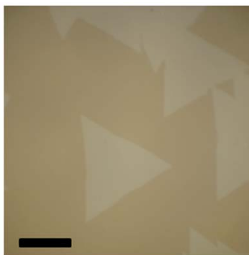
Figure 3.2 Optical micrograph of a monolayer WSe 2 on sapphire substrate Scale bar corresponds to 25 \mu\text{m} .
