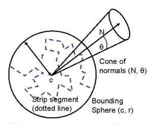
**Fig. 9** Information associated to each segment of the triangle strip: Centroid of all vertices (c), bounding sphere radius (r), average face normal (N) and radius of the cone that contains all normals  $(\theta)$ .
