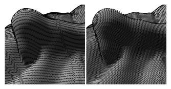
**Fig. 6** Any weighing scheme can be used to indicate the preference for a particular type of single-strip. In the first figure (**left**), horizontal edges of the head model were assigned a high weight, while in the second figure (**right**), vertical edges were similarly penalized. The results are single-strips with different general orientation.
