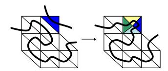
**Fig. 8** Removing outgoing peaks from a cluster of triangles. The identified outgoing peak (in dark on the left figure) is split, together with an adjacent triangle inside the cluster. After the operation, no triangle in the resulting cluster has two boundary edges, and it is possible to reduce the number of times the strip crosses a cluster boundary (indicated with a thick black line).
