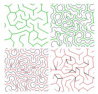
Fig. 12 Left to right and top to bottom: (a) Spanning tree of mesh edges, used to produce strips with low cache-miss ratio. Edges in the tree receive positive weight, and the rest get weight zero. (b) The produced single strip is superimposed on the spanning tree. (c) We substitute the spanning tree with the medial axis of the single strip. (d) Dark edges highlight the few differences between medial axis from 'c' and spanning tree from 'a'.
