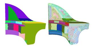
Fig. 7 (a) Left: Triangle clustering based on normal deviation. Triangles in the same cluster are shaded with the same color. Clusters minimize the normal deviation among the triangles contained. (b) **Right**: Disjoint triangle strip loops before merging. The weight maximizing edge matching produces strips that hardly cross the cluster boundaries.
