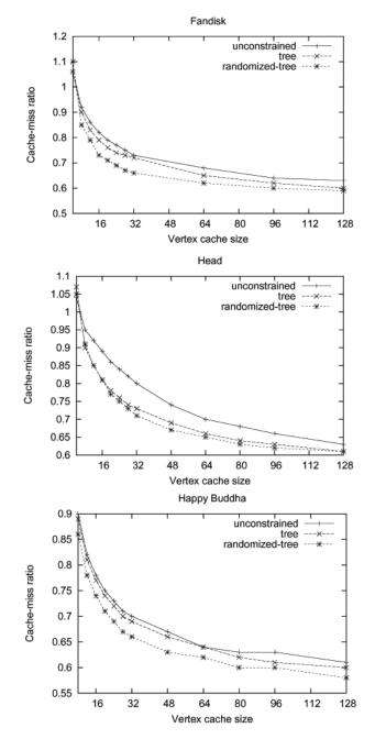
**Fig. 15** Cache-miss ratio for the single-strips of three models (Fandisk, Head and Happy), obtained in three different ways: Unconstrained strips, with the spanning tree method, and with the randomized spanning tree method. In all cases, the randomized version of our optimization performs better. Notice the specially large difference for the popular cache sizes of 16 and 32 vertices.
