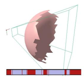
**Fig. 11** Real time back-face culling in the sphere model. The bar indicates rendered parts of the single-strip, which are rendered, in dark color, and culled parts in light color. The high spatial coherence observed in the single-strip allows culling many triangles with few cuts.
