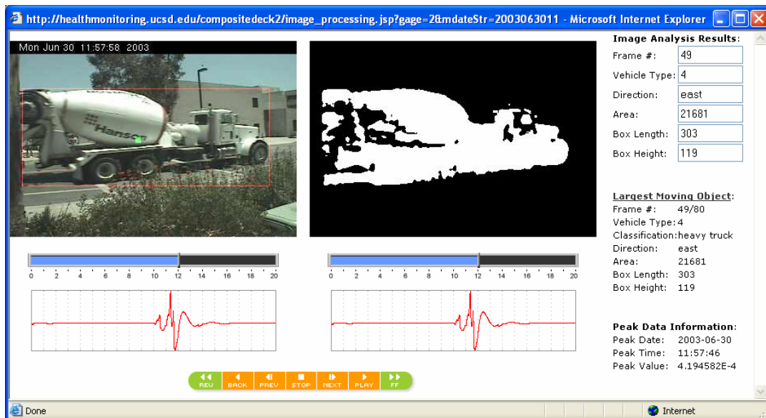
Figure 4.24: Example of Data Fusion of Recorded Strains, Recorded Video, and Extracted Features for a Concrete Truck
