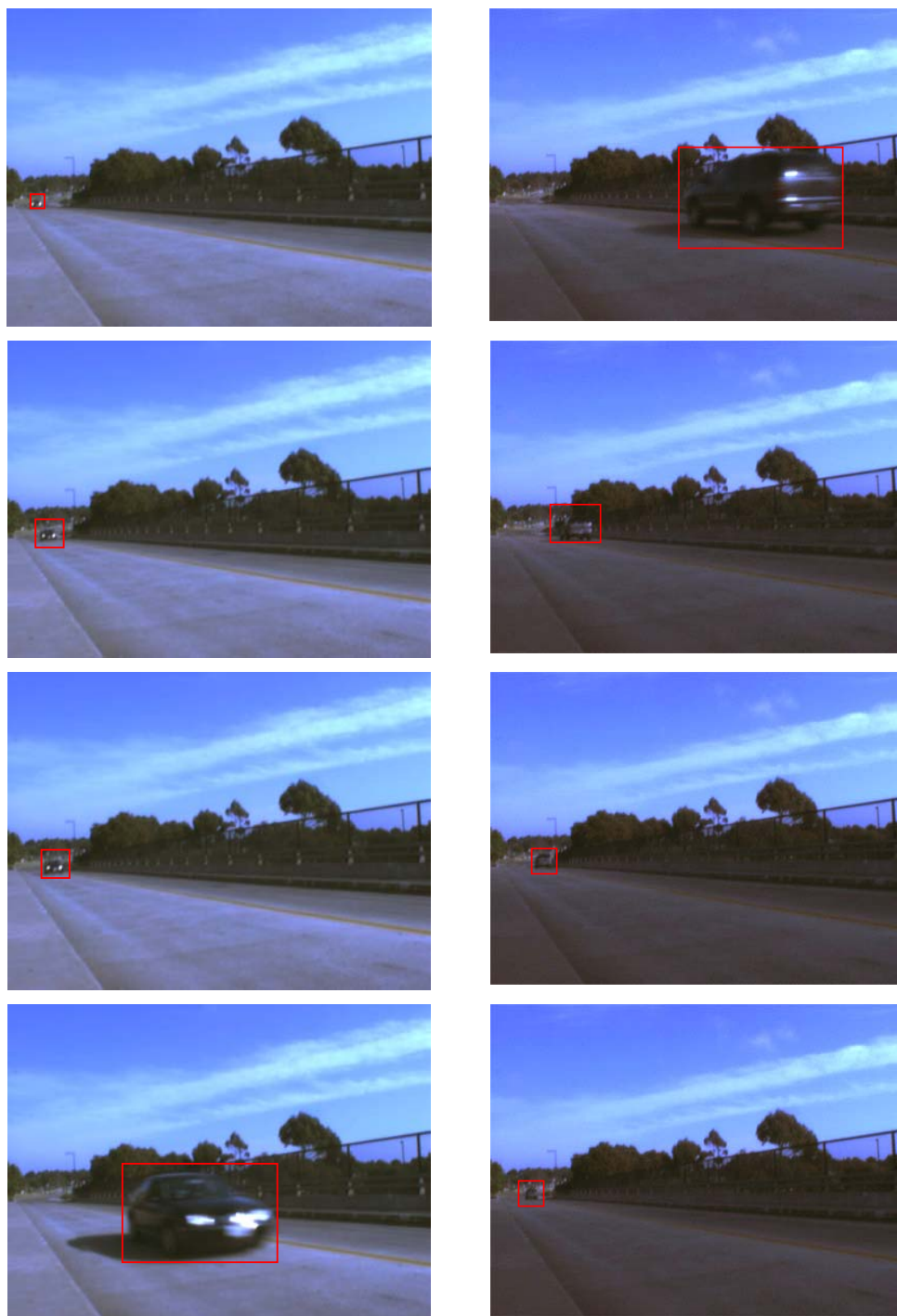
Figure 9.24: Recorded Images for 2 Typical Cars Taken when the Vehicle Reaches Channels 8, 6, 3, 1 (Top to Bottom).
