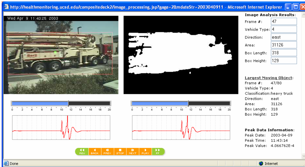
Figure 4.22: Example of Data Fusion of Recorded Strains, Recorded Video, and Extracted Features for a Large Multi-Axle Truck
