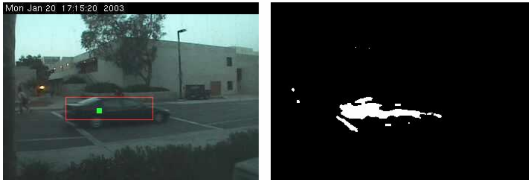
Figure 4.14: Original and Processed Image with Only Partial Detection and Gaps Resulting From Insufficient Resolution
