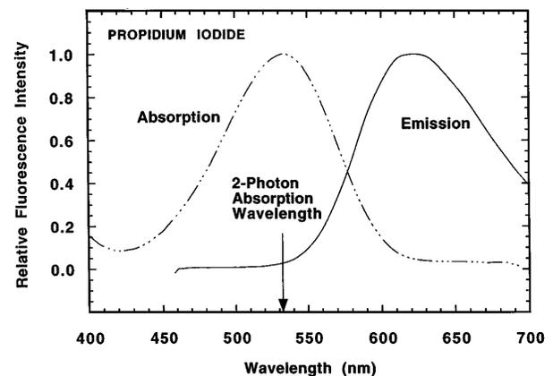
Fig. 1. Measured absorption and emission spectra for the fluorescent dye PI bound to DNA. Fluorescence emission is excited in a dye-tagged human sperm cell by a two-photon absorption process while the sample is held in 300-mW, 1064-nm cw optical tweezers.
