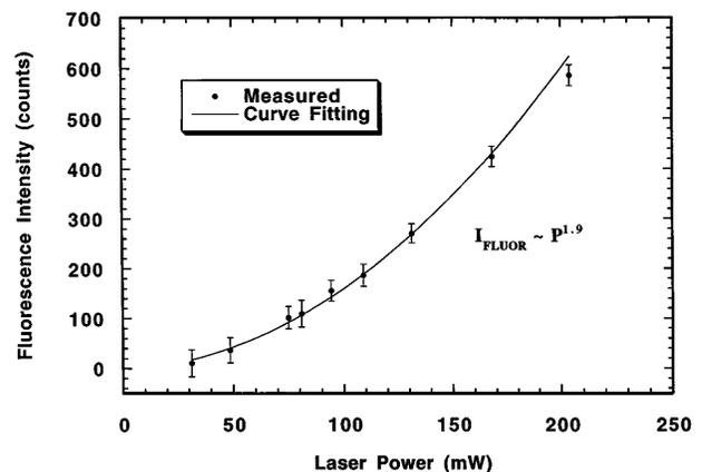
Fig. 2. Dependence of PI fluorescence intensity ( $I_{\text{FLUOR}}$ ) on trapping (pump) laser power. The intensity varies with nearly a square-law dependence on incident laser power ( $I_{\text{FLUOR}} \sim P^{1.9}$ ). The CCD integration time was 5 s.
