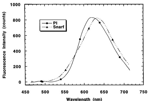
Fig. 4. Two-photon fluorescence emission spectra for two different CHO's that have been tagged with PI and Snarf.
