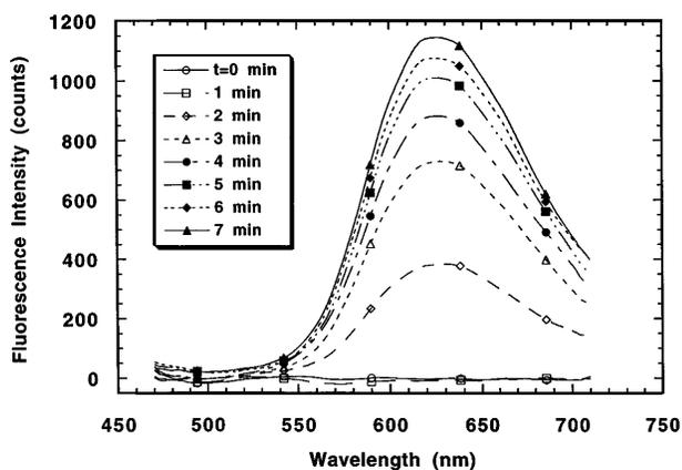
Fig. 3. Time dependence of fluorescence intensity, measured for an optically trapped human sperm cell that is held stationary for 7 min in a 300-mW optical trap.
