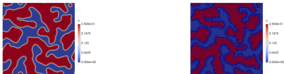
Fig 6.4 Phase field model for a \text{UO}_2 - \text{U}_4\text{O}_9 microstructure evolved at 400 K and an initial concentration of oxygen of 0.20. (b) Meshed microstructures showing refinement of the quadrature points on the mesh with a high concentration of points capturing the interface between the two phases.
