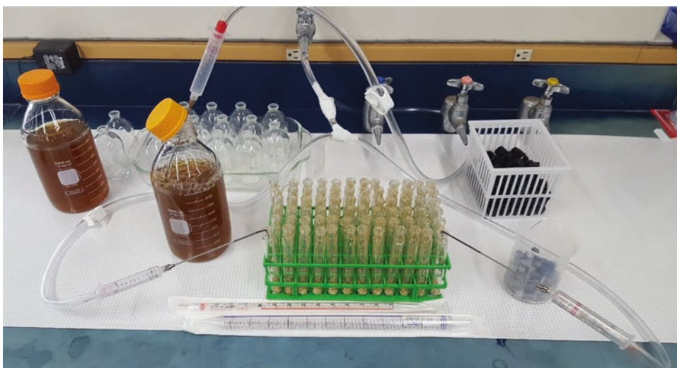
Fig. 1 Media dispensing setup with a three-way gas manifold (clear-colored) to supply carbon dioxide simultaneously to the media bottle and two Hungate tubes to be filled. Also shown: a rack of Hungate tubes with prealiquoted plant material (center); two 1-L bottles of Medium C (left); serological pipets used for dispensing medium (center); black caps and grey butyl rubber septa for sealing Hungate tubes after medium is dispensed (right)
