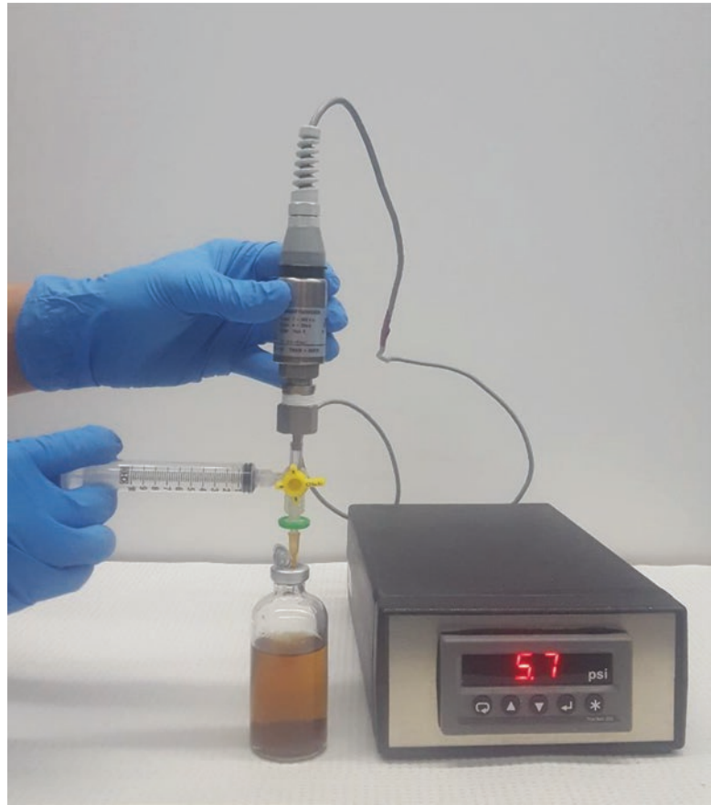
Fig. 2 A pressure transducer assembly with digital display is used to measure the accumulation of gas pressure in the headspace of a fungal culture in a 60-mL serum bottle
