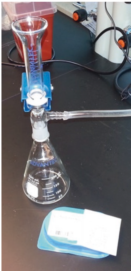
Fig. 1 Vacuum filtration apparatus. A membrane filter equipped with a vacuum filtration apparatus can harvest biomass quickly with minor metabolism changes during the sample handling
