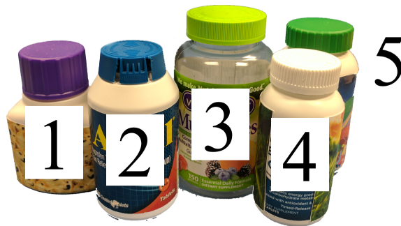
Figure 4.1: Bottles used in experiments. (1) bottle with push-and-twist safety mechanism. (2) bottle with pinch-and-twist safety mechanism. (3) bottle with push-and-twist safety mechanism. (4) bottle with push-and-twist safety mechanism. (5) bottle with no safety mechanism.
