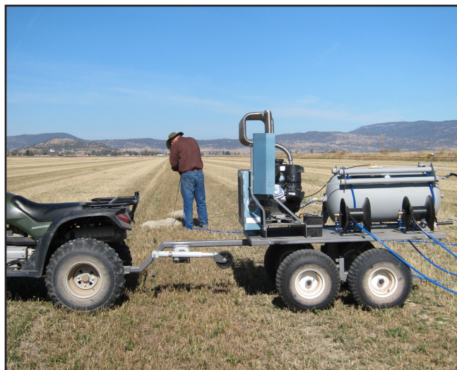
Figure 1. Pressurized exhaust device (PERC) used to evaluate pocket gopher and Belding's ground squirrel control.
