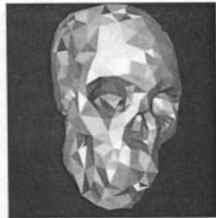
Figure 12: The skull data set at level-of-detail 29 contains 2,428 triangles. The mesh along with the collapsing triangles and their stencils are shown.
