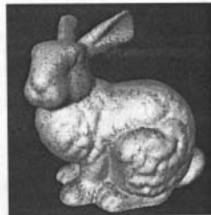
Figure 13: The original bunny data set contains 69,668 triangles. The mesh along with the collapsing triangles and their stencils for this initial level are shown.
