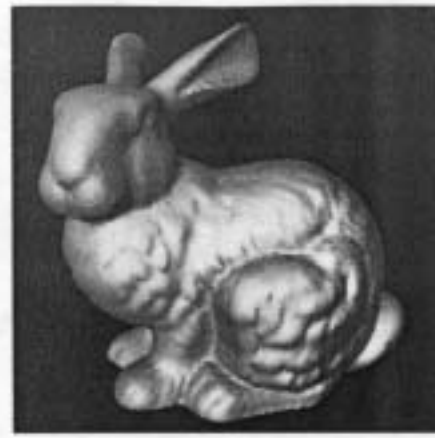
Figure 17: The original bunny data set using flat shading. The data set contains 69,668 triangles.
