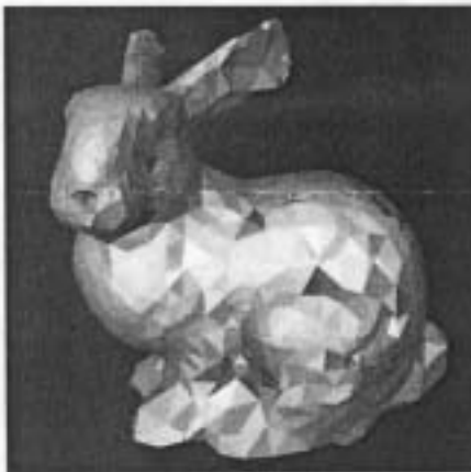
Figure 16: The bunny data set at level-of-detail 25.67 contains 4,944 triangles, some of which are partially collapsed. The mesh along with the collapsing triangles and their stencils are shown.
