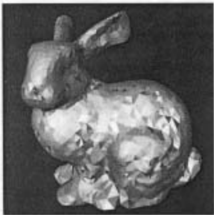
Figure 15: The bunny data set at level-of-detail 18.95 contains 10,408 triangles, some of which are almost completely collapsed. The mesh along with the collapsing triangles and their stencils are shown.
