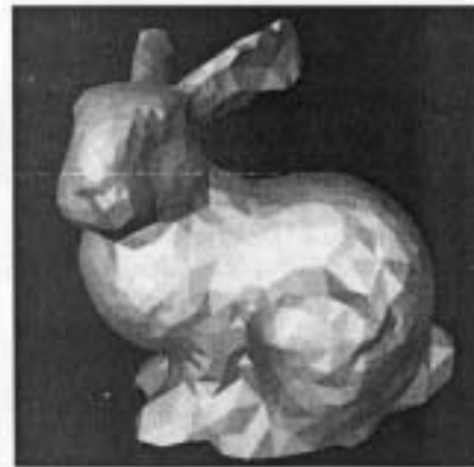
Figure 19: The bunny data set at level-of-detail 25.67 using flat shading. The mesh contains 4,944 triangles.
