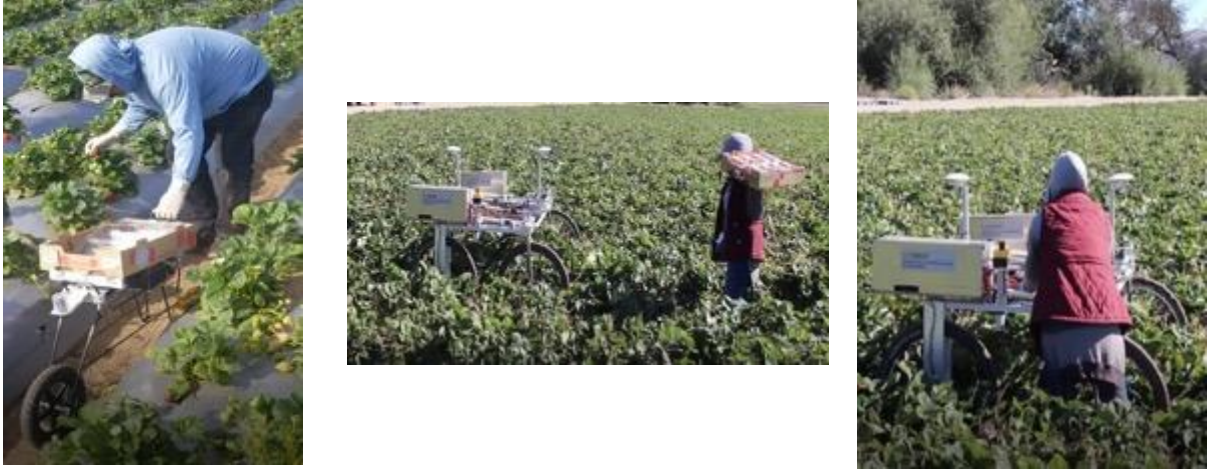
Figure 2. The working cycle of co-robotic harvesting in an open commercial field: a) the picker is picking strawberries inside the furrow in the same way as the manual harvesting; b) the picker walks a small distance to the serving robot; c) the picker loads the trays on the robot;
