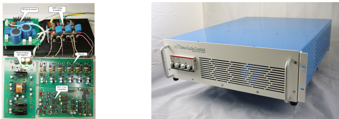
Figure 1: UCI EISG OCC-APF (left); OCC-APF for PIER Field Demonstration (right)
