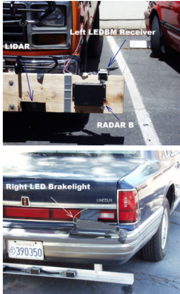
Figure 3. Mounting of LEDBM System and Test Components
