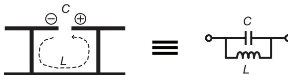
Figure 1.5: The unit cell of a periodic structure is usually a resonant circuit. The shorted-patch-based impedance surface unit cell is used here as an example. At resonance, the charges are collected in the adjacent patches in the gap. The path from one patch to another through the vias constitutes the current path, forming an inductor.
