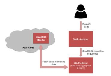
Figure 4.3: Cerebro architecture and component interactions.
