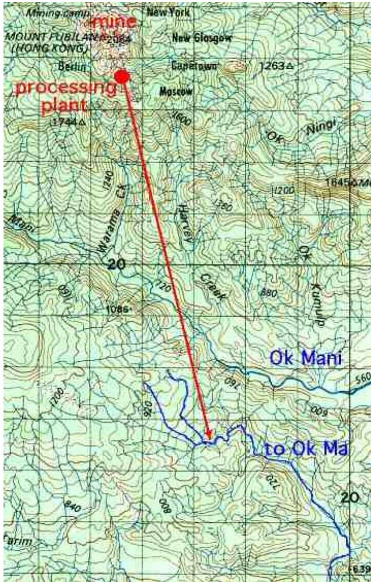
Figure 5. Tailings pipeline beginning and terminal points from 1996 proposal (Kehdingen, 2001).
