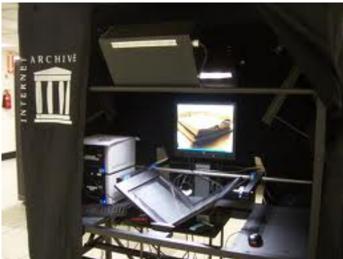
Figure 5: The Internet Archive’s Scribe image capture machine. Photograph courtesy of Internet Archive.
