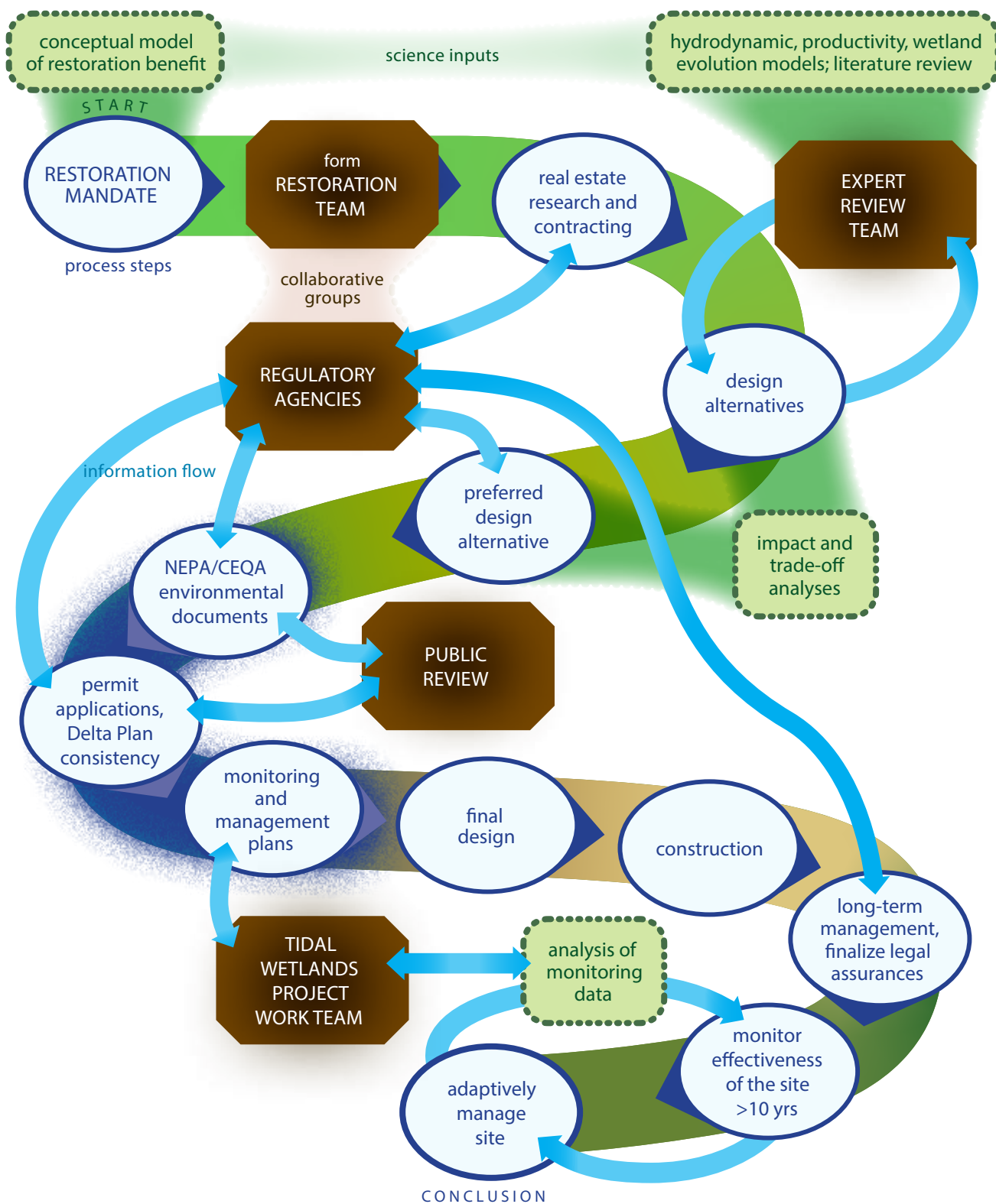
Figure 2 Steps in the process of constructing and evaluating tidal wetland restoration sites for fish. CEQA: California Environmental Quality Act; NEPA: National Environmental Protection Act.
