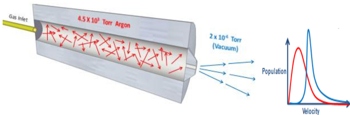
Figure 2.4: High pressure argon gas is expanded into a vacuum through a small nozzle. Random thermal motion of the argon molecules (red arrow) is converted into directed kinetic motion (blue arrow). This results in a low translational temperature (around 1K) which in turn leads to a narrow velocity distribution due to the fact that the width of the velocity distribution is a direct measure of the translational temperature of the gas.
