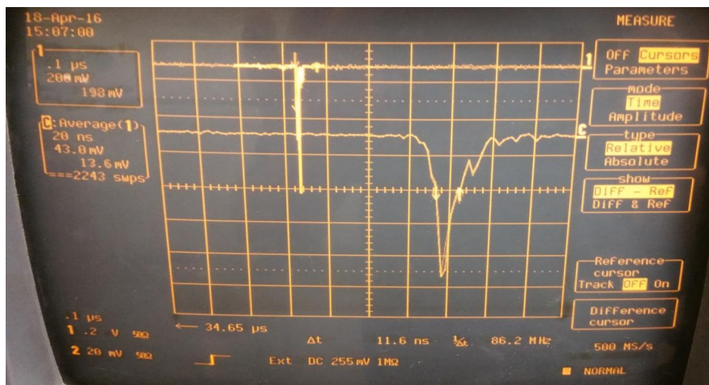
Figure 2.24: Average signal of theophylline (bottom trace, labeled C) and instant signal from channel 1 at 10 Hz (top trace, labeled 1). Two cursors on the average are set to measure the FWHM of the mass peak which is ~ 12nsec wide and the average signal is ~200 mV.
