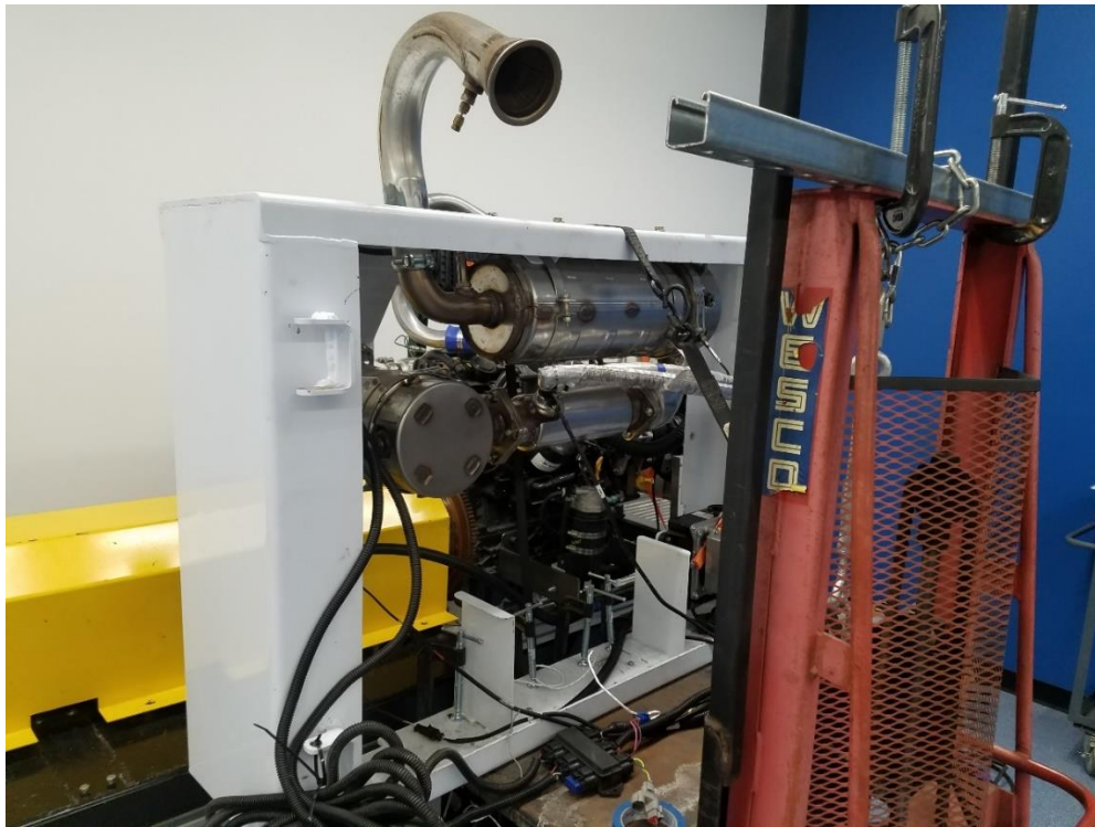
Figure 7-5 Mini-Excavator Engine on the Engine Dynamometer with the DPF
