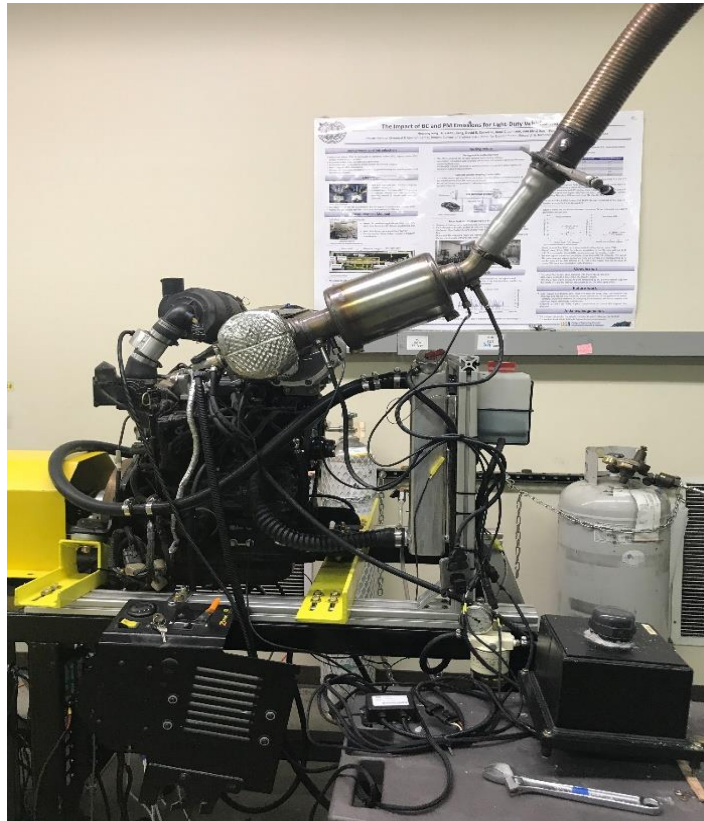
Figure 7-3 Ride Mover Engine on the Engine Dynamometer with the SCR
