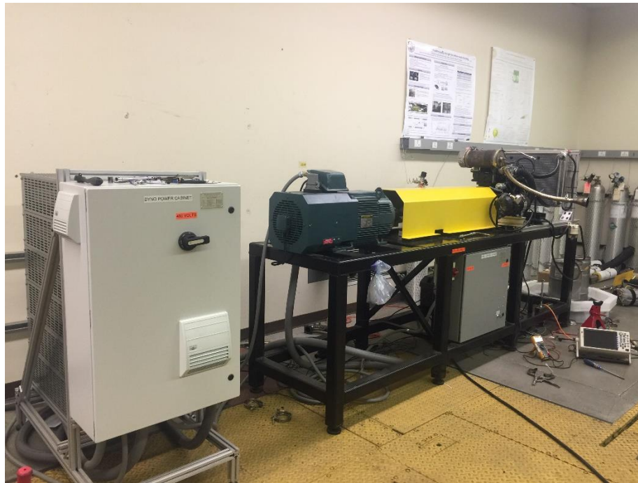
Figure 7-6 Engine Dynamometer used for Testing
