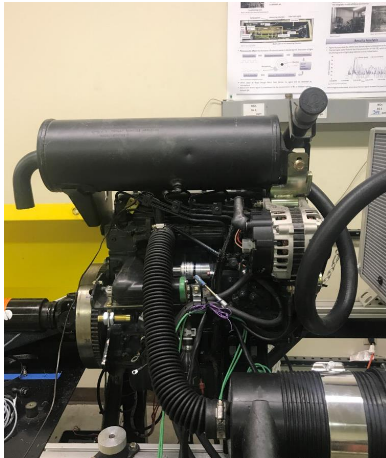
Figure 7-4 Mini-Excavator Engine on the Engine Dynamometer with the DPF
