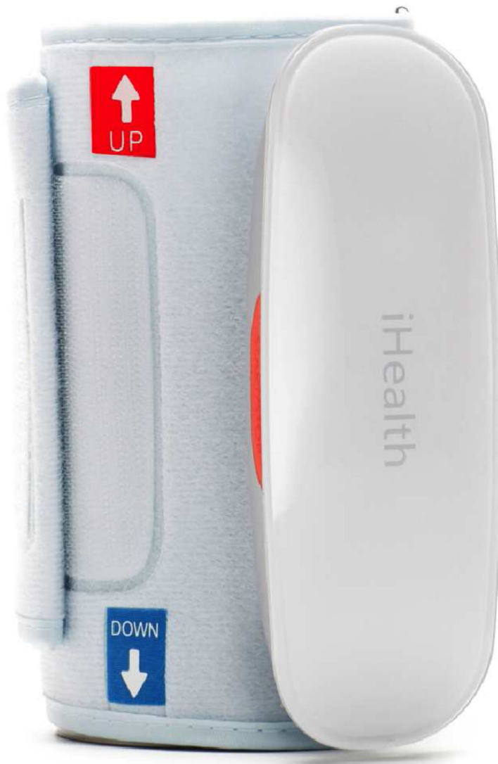
Figure 7. Left: Photograph of an iHealth BP5 wireless blood pressure cuff. The cuff firmware is modified to allow users to execute the cFMD measurement protocol. Right: Measurement application running on an iPhone 5 that obtains the pressure waveforms from the cuff via Bluetooth.
