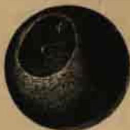
FIG. 298.—Black Spherule with Metallic Nucleus (?). This spherule, covered with a coating of black shining magnetite, represents the most frequent shape. The depression here shown is often found at the surface of these spherules. From 2375 fathoms, South Pacific.
