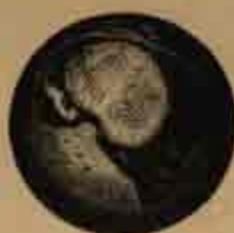
FIG. 299.—Black Spherule with Metallic Nucleus (?). The black external coating of magnetic oxide has been broken away to show the metallic nucleus, represented by the clear part at the centre. From 3159 fathoms, Atlantic.
