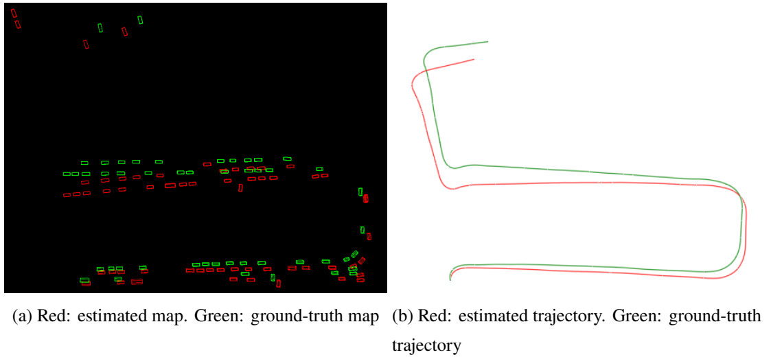
Figure 7.5: Visualization of estimated ground-truth semantic map and input camera trajectory for sequence 07.
