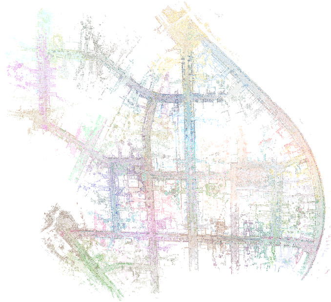
Figure 3.6: KITTI scene fragments visualization. We merge every k = 50 consecutive LiDAR frames into a scene fragment. Then these scene fragments are transformed to the world frame with the ground-truth trajectory. Each color represents a scene fragment.
