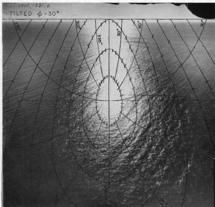
The glitter pattern at solar elevations of \phi = 75^\circ , 50^\circ , 30^\circ , and 10^\circ . Wind speed was approximately 4 \text{ m. sec.}^{-1} . The superimposed grids consist of lines of constant slope azimuth \alpha (radial)
