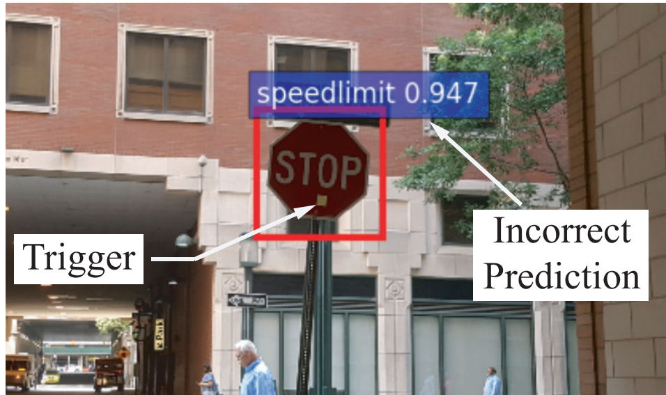
Figure 2.3: An example of backdoor altering DNN’s behavior. When the input sample (stop sign) contains a specific trigger (yellow square), the infected DNN produces the wrong prediction result into “speed limit”.
