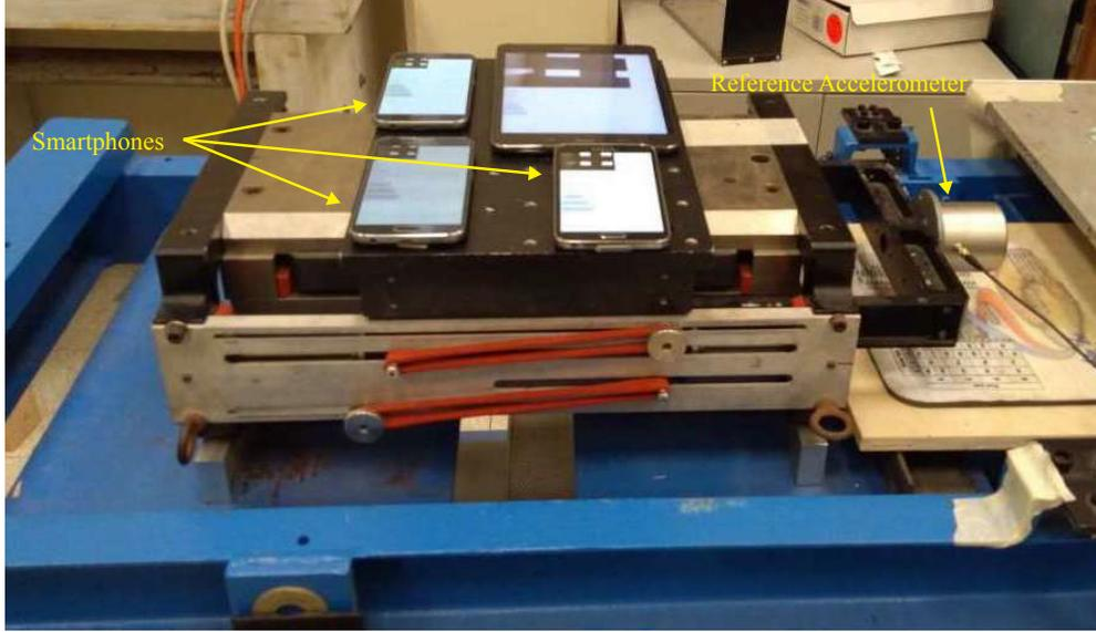
Figure 4.6: Shake table experimental setup. The reference accelerometer (Model393C [1]) was attached to the shake table, which is shown on the right hand side.
