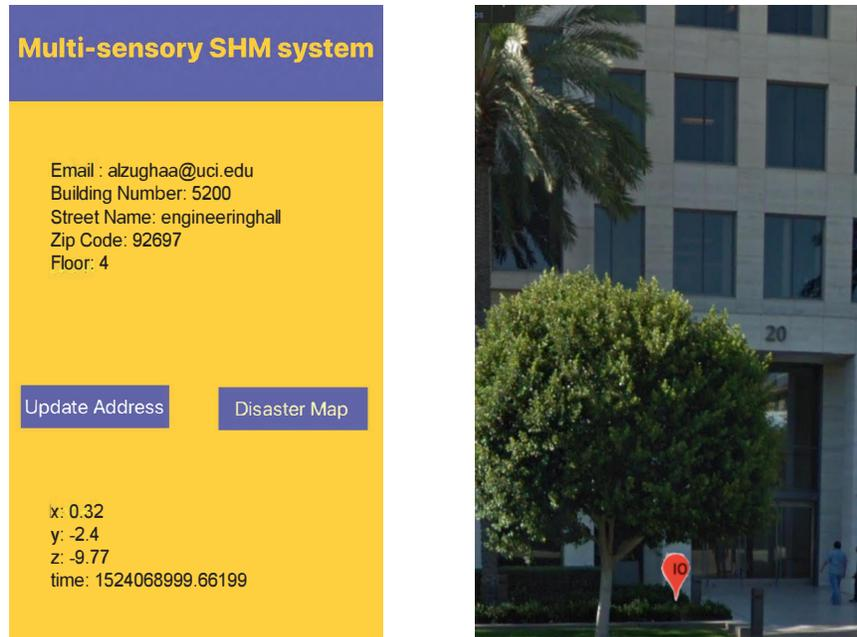
Figure 4.3: Screenshots of the smartphone application. The seismic sensing is performed silently in the background. The building’s structural safety status is fed back to the user in the form of a disaster map.
