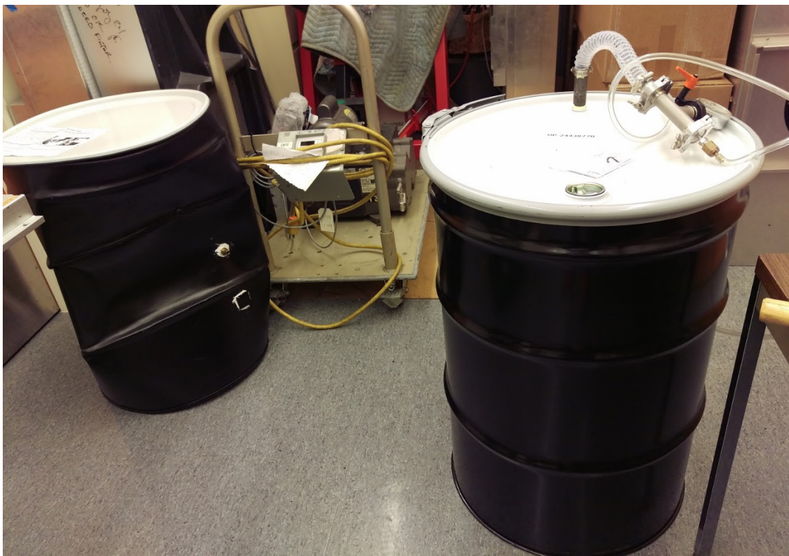
Figure 63: Steel drum CVD test for silanization.
