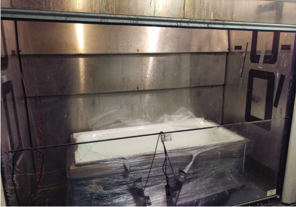
Figure 60: Scaled hydrothermal bath setup with a ceramic, insulated tub for processing.
