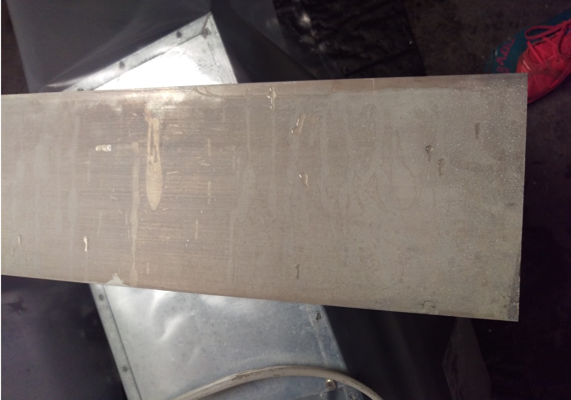
Figure 62: Test coupon of aluminum sheet metal to verify ZnO coating.
