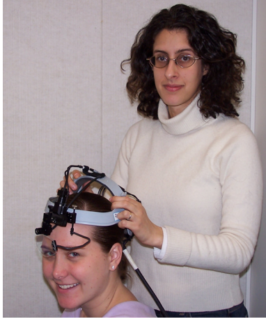
Figure 1: Volunteer modeling the ASL head-mounted eye-tracker that participants wore during the experiment. The eye-tracker recorded the position of the participant’s gaze.
