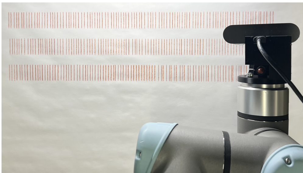
Figure 5.3: Overhead view of Ur5e robot performing line strokes.
