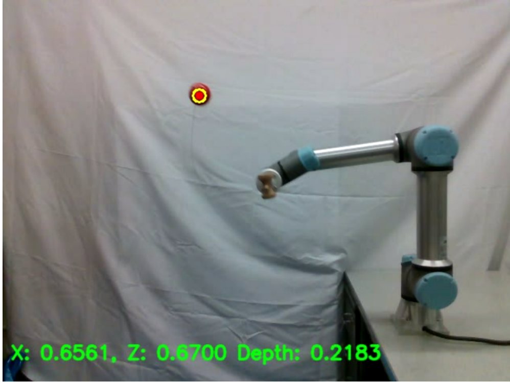
Figure 2.3: Video feed from the depth camera during the catch phase of the experiment.
