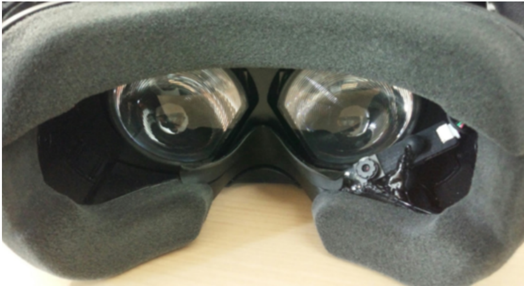
Figure 4.1: Eye tracking camera setup. Pupil Labs eye trackers were installed in an HTC Vive headset.
