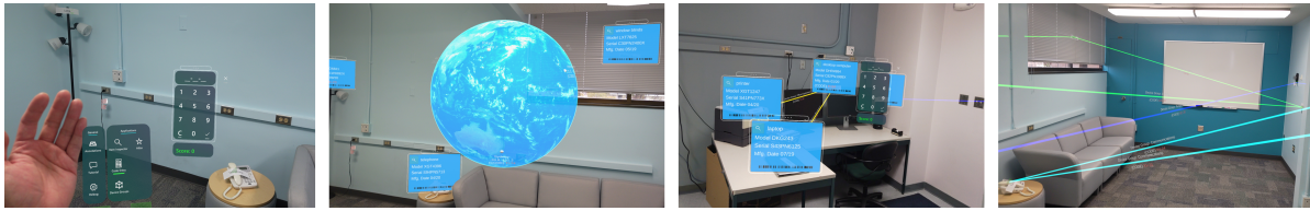
Figure 7.1: Images of the Layerable Apps paradigm showing (left to right) Code Entry and the Application Switcher, Atlas, Item Inspector, and Device Groups, all of which can be displayed concurrently to facilitate passing of information among them. In experiments, users were required to switch between and integrate information from all apps using different methods of application selection.
