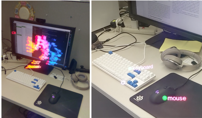
Figure 5.3: Left: Raw points returned from object recognition as projected into 3D space, accumulated over several frames. This shows the variance in predicted positions and false positive label predictions. Right: Scene correctly labeled with object-permanent labels.
