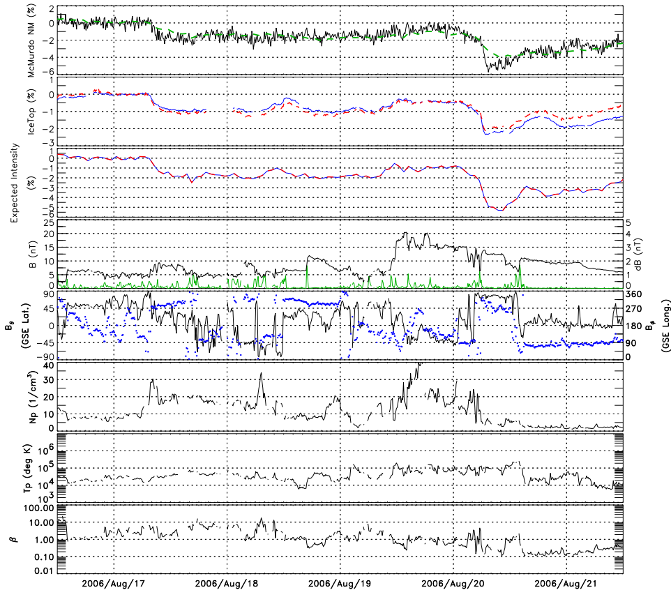
Figure 4: August 17-21, 2006. From top: (1) McMurdo monitor (black) and Spaceship Earth isotropic component (green dashed). (2) IceTop SPE (blue) and MPE (red dashed) scaler rate, 32 DOM average. (3) IceTop model prediction. (4) Interplanetary magnetic field magnitude (black) and derivative (green). (5) Field direction latitude (black) and longitude (blue dots). (6) Plasma density. (7) Plasma temperature. (8) Plasma \beta .
