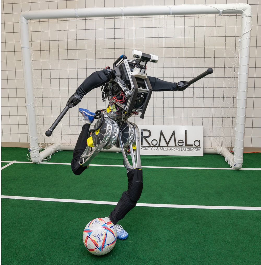
Figure 2.1: ARTEMIS, a next-generation humanoid designed for dynamic and agile motions.
