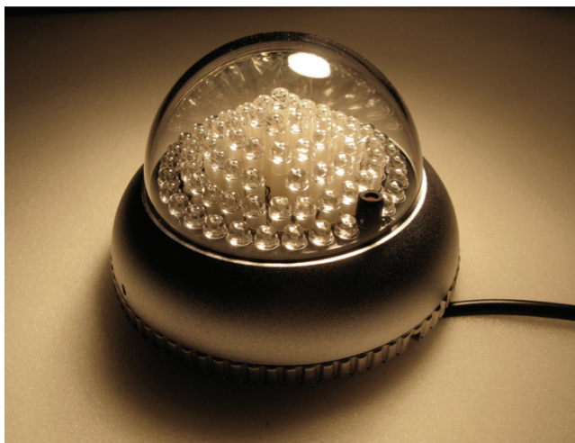
Figure 5. Infrared dome illuminator LIR-CA60. Infrared light can be seen by specially equipped video cameras commonly used in surveillance and military applications. Infrared cameras can “see in the dark” images otherwise invisible to the human eye.
