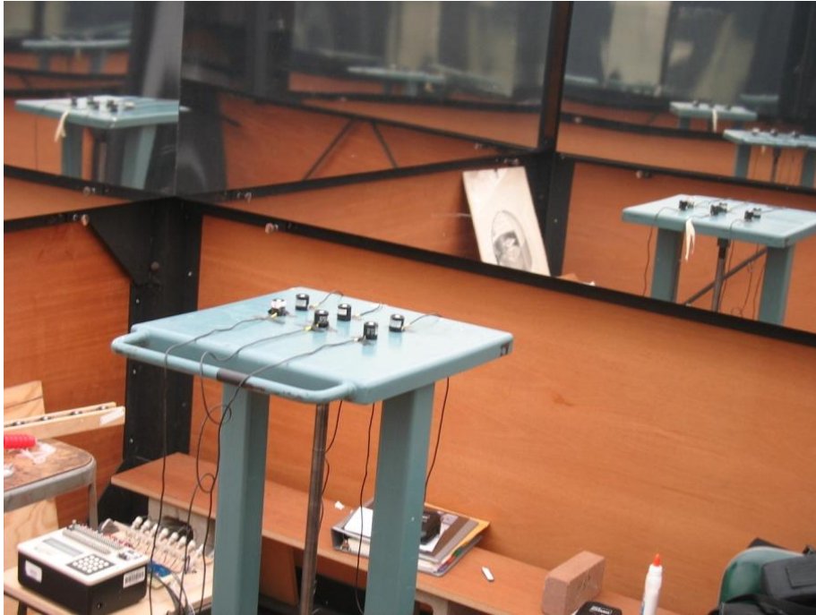
Figure 41 LI-COR photometric sensors in overcast sky simulator
