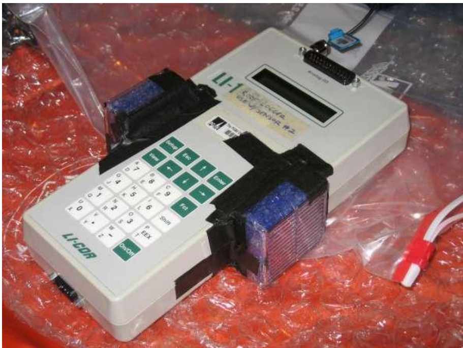
Figure 42 LI-COR LI-1400 data logger
