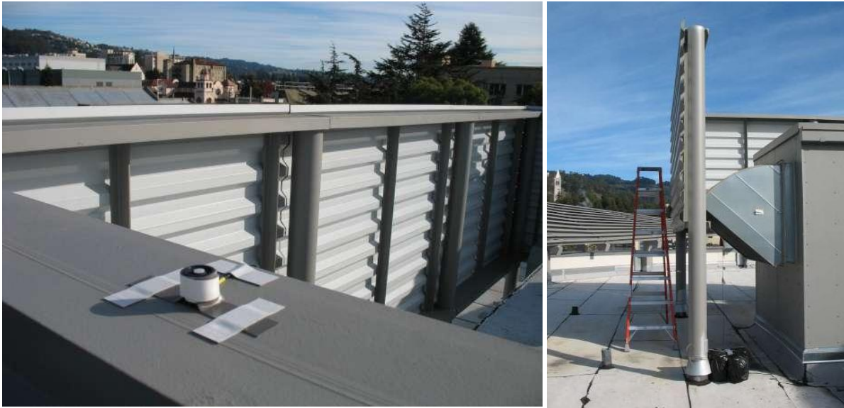
Figure 43 (left) Sensor used to measure global horizontal illuminance
