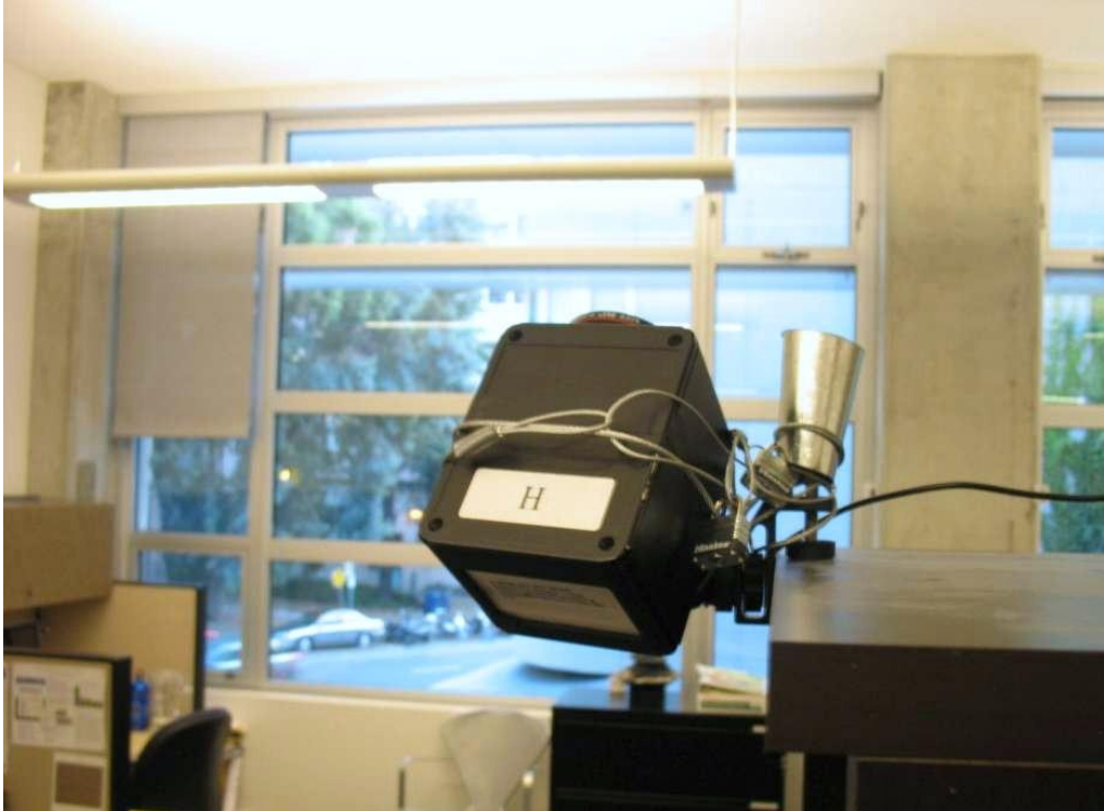
Figure 37 Fisheye lens camera used for monitoring shade and lighting control
