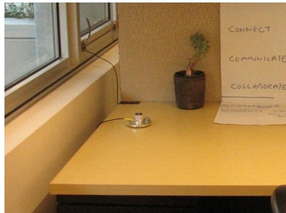
Figure 40 LI-COR LI210SA photometric sensors mounted at workstation #3 (left) and workstation #4 (right)
