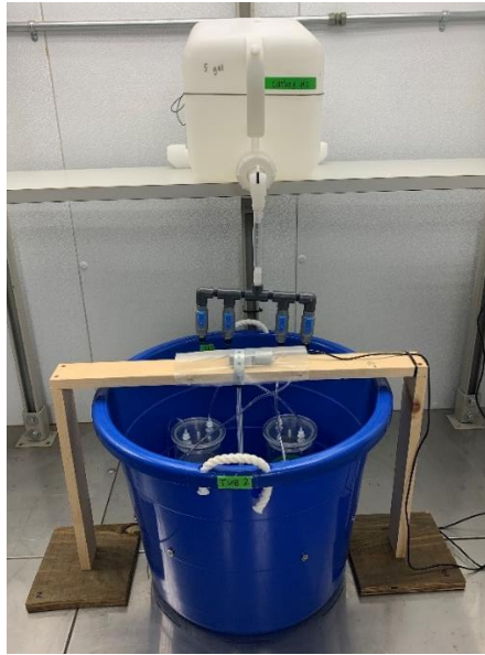
A7 Incubation chamber set-up. A single incubation chamber set-up, fit with (1) 4-way valve unit, (2) soil and blank cores fitted with magnetic spinning lids, and (3) central magnetic stirring unit connected to motor box. Note the motor box is not pictured.
