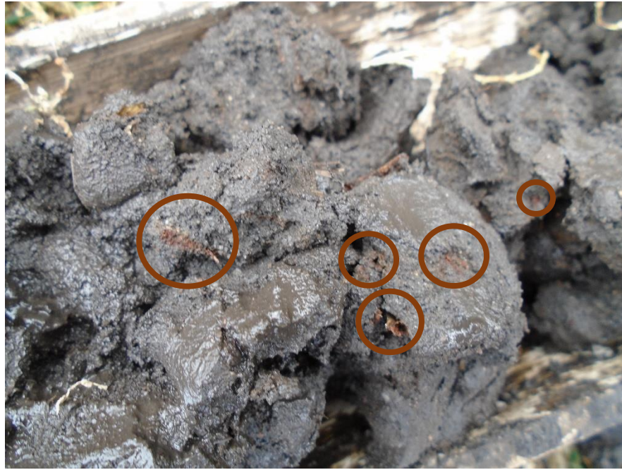
Figure 2-S4 Fe concretions among a reduced soil at the upper wetland position of Cowell Ranch. Fe concretions were identified between 20 and 110 cm depth below ground, indicative of wetting and drying induced by surface water presence and absence (e.g. tides, precipitation).
