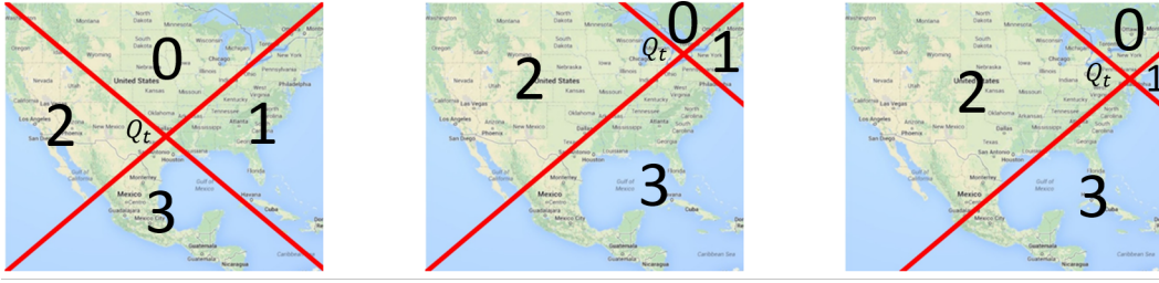
Figure 5.4. A 2-dimensional version of the BSC BCI described in Section 5.1.2. At every time step, the query point Q_t is updated based on user responses, and as such, so are the dividing lines. The large numbers simply represent indices for identifying each quadrant.
