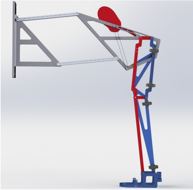
Fig. 17: The parallelogram mechanism attaches to the six-bar linkage in order to control the foot orientation angle.
