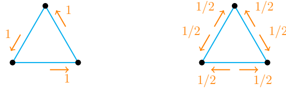
Figure 6.3: A graph with 3 vertices and three edges and two different balanced allocations with zero baseload. Note that the total load at each vertex is the same for the two allocations and is equal to 1 at each vertex.
