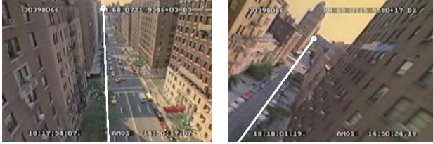
Figure 8: Extracted vanishing point pairs (a white line segment connects the two vanishing points).
