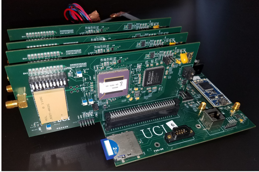
Figure 1.3: 2011 Data acquisition core prototype using ATWD
