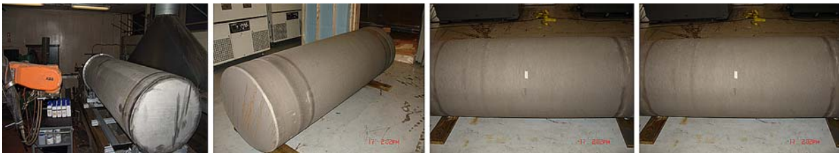
Fig. 10—Effect of GM9540P salt-fog test on HVOF coating of SAM1651 amorphous metal on a half-scale SNF prototypical waste package.
