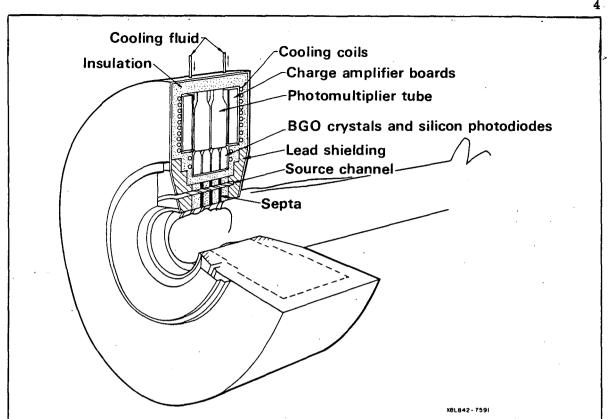
Figure 2: Cooled tomograph gantry for keeping silicon photodiodes and charge amplifiers at a reduced temperature (typically -30°C).
