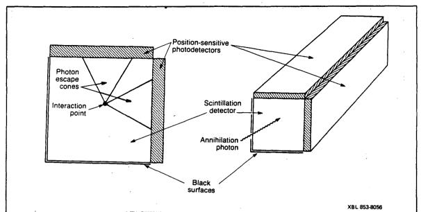
Figure 3: Detector module consisting of a rectangular scintillation crystal and photodetectors capable of determining the location of the interaction point within the crystal.
