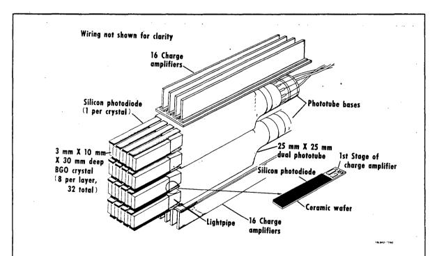
Figure 1: Multi-ring detector array where groups of 8 crystals are coupled to a common phototube for timing information and coupled individually to silicon photodiodes for the identification of the crystal of interaction. Square phototube (Hamamatsu R1548) has two independent electron multipliers and first stage of charge amplifier is mounted near photodiode.
