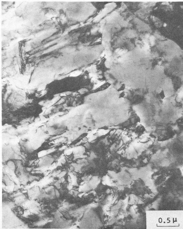
Fig. 8. Transmission electron micrographs of a heat treated Fe-8Ni-2Mn-0.25Ti alloy. (a) Bright field image showing substructure. (b) Dark field image from the (200)_{\gamma} reflection. The bright areas in the dark field image are properly oriented austenite grains.
