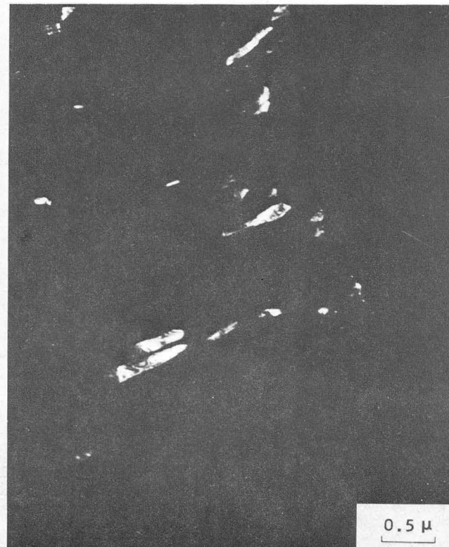
Fig. 8. Transmission electron micrographs of a heat treated Fe-8Ni-2Mn-0.25Ti alloy. (a) Bright field image showing substructure. (b) Dark field image from the (200)_{\gamma} reflection. The bright areas in the dark field image are properly oriented austenite grains.
