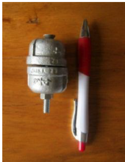
Figure A3 SUM holder designed to encase the stove use monitor to protect it from malfunctions when exceeding temperatures of 85 degrees Celsius
