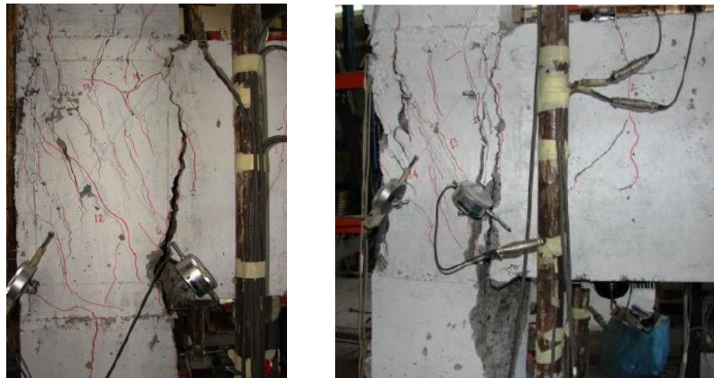
Figure 3.28 Specimens US3-C-Control and US3-CS-Control failure modes, Topcu [143]
