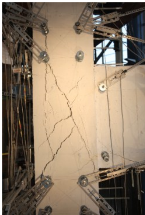
Figure 7.25 (Continued) North joint face crack development and progression during EW beam loading of specimen U-J-2
