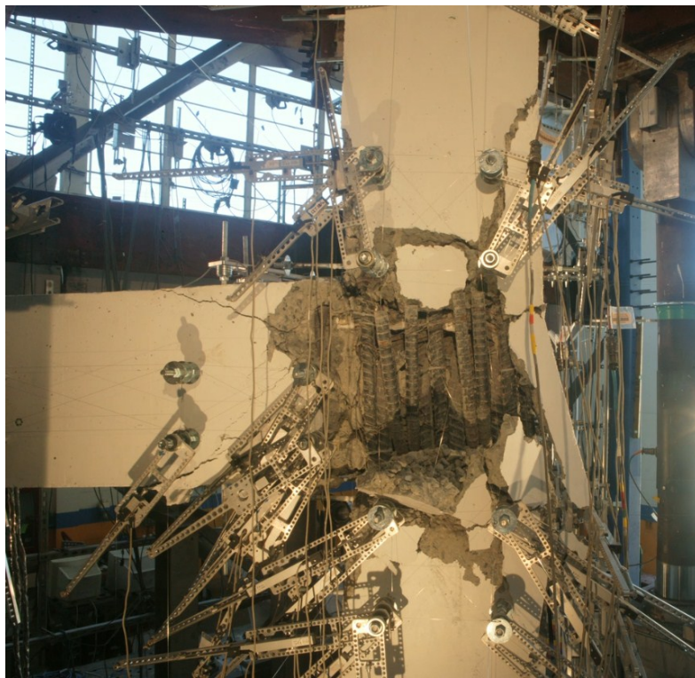
Figure B.7 East joint face instantly before axial failure of specimen U-J-1
