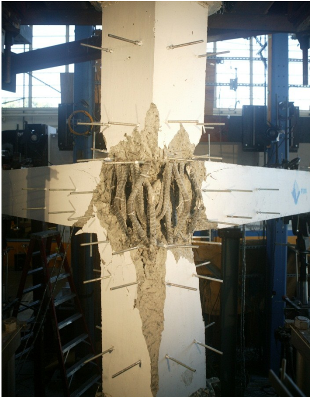
Figure 7.48 Global views of Specimen B-J-1 axial collapse
