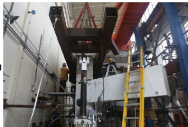
Lateral restraining frame
