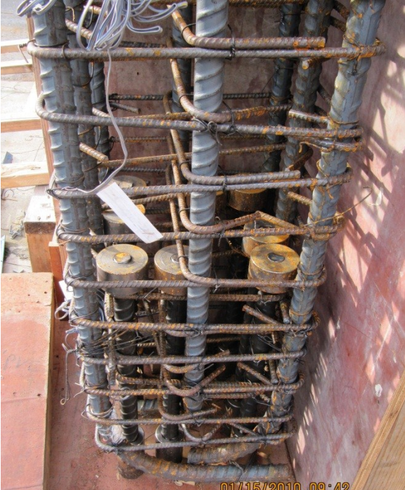
Figure 6.8 Reinforcement cage of specimen U-J-2
