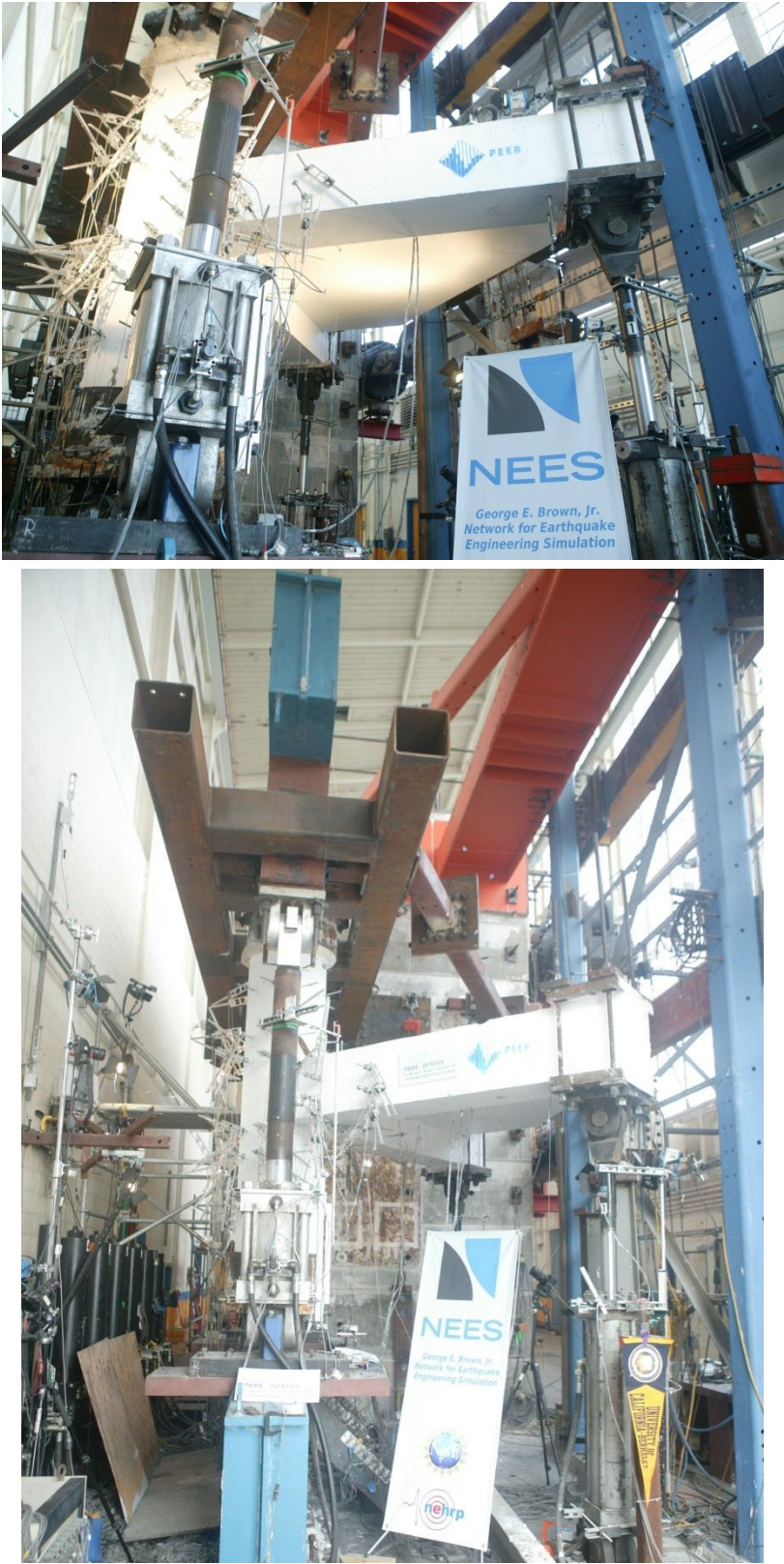
Figure 6.35 Specimens B-J-1 and U-BJ-1 in the test rig.
