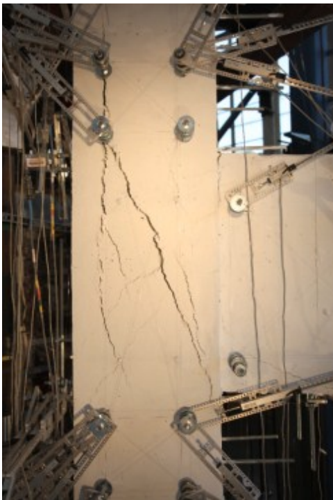
Figure 7.25 (Continued) North joint face crack development and progression during EW beam loading of specimen U-J-2
